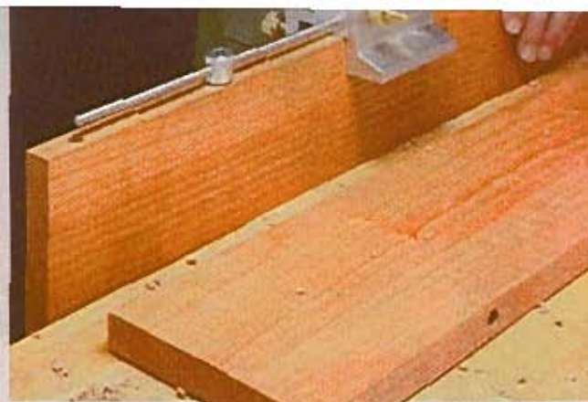
▲ Edge Joints. The distance gauge is used to accurately space dowel holes in edge joints.
