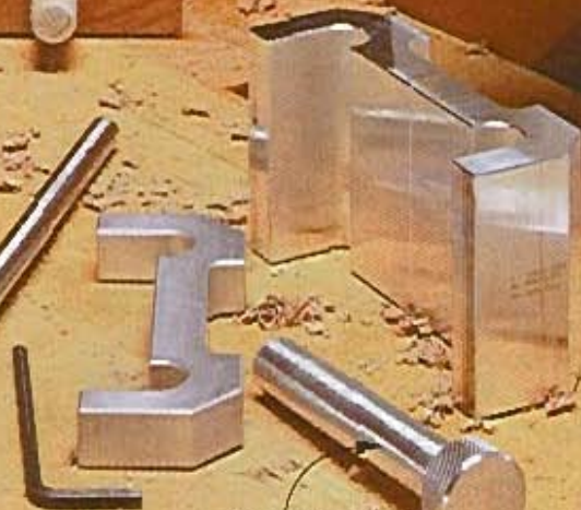
Jig can be repositioned quickly with indexing pin
