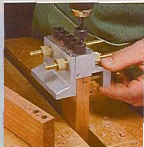
▲ Matching Holes. To drill matching holes in the end of the mating piece, you repeat the process. The jig is clamped flush with the marked edge of the workpiece.
