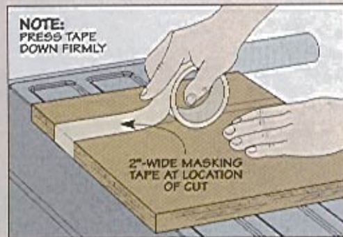
▲ Tape Reinforcement. Masking tape pressed firmly onto the workpiece will reinforce the wood for a chip-free cut.
