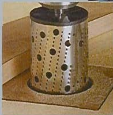
▶ Power Shaper. A Microplane drill press rotary shaper cuts faster than a drum sander and won't clog or burn the workpiece.
