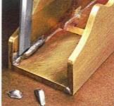
▲ Cleaning the Inside. An old chisel comes in handy to remove any globs of solder from inside the body of the plane. Then you can scrape or sand away any remaining traces.
