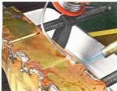
▲ Soldering. One of the keys to successful soldering is to heat the metal until the solder just begins to flow into the joints.
