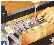
Adjust the Fingers. Using the tail board as a guide, adjust the fingers to match nearly any layout you can come up with.
