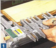
The Initial Setup. Even though you'll rout the tails to start with, the first step is to install the finger assembly in the "PIN" position.
