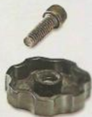
▲ Locking Knob. To make the locking knob for the layout square, a cap screw is press-fit into a blind hole in the center of the knob.
