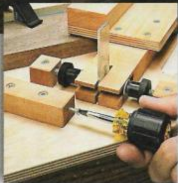
▲ Fine Tuning for a Perfect 45° Cut. With the guide assembly at 45°, set the screw until it touches the aluminum stop (see insert). Then it's easy to return to this position by just flipping the stop down and adjusting the knobs.
