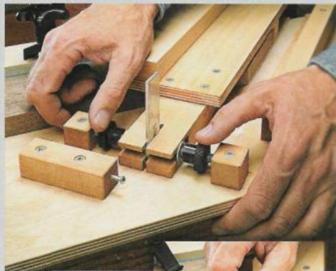
▲ Plus or Minus 45° Cuts. Whenever you need to cut an angle greater or less than 45° to square up a miter joint, simply lift up the aluminum guide stop. Then adjust the two knobs to change the miter angle for trimming.
