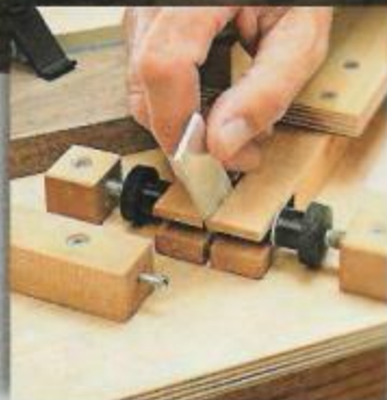
▲ Plus or Minus 45° Cuts. Whenever you need to cut an angle greater or less than 45° to square up a miter joint, simply lift up the aluminum guide stop. Then adjust the two knobs to change the miter angle for trimming.
