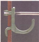
▲ Spread Your Wings. Push the screw in to spread the wings behind the pegboard and lock in the hook.
