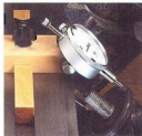
▲ Read the Runout. A dial indicator is an accurate method for checking the runout of the table saw arbor (top) or flange (bottom).
