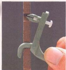
▲ Insert Hook. With the white, nylon screw backed out, slip the hook into a pair of holes in the pegboard.
