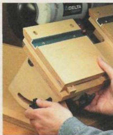
▲ Pivot. To adjust the angle of the pivoting platform, loosen the two star knobs on the sides of the wings and swing the platform into position.
