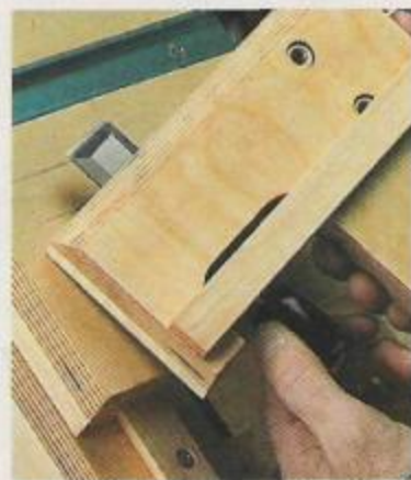
▲ Check Your Progress. You can check your grinding progress by simply turning the tool sled over.
