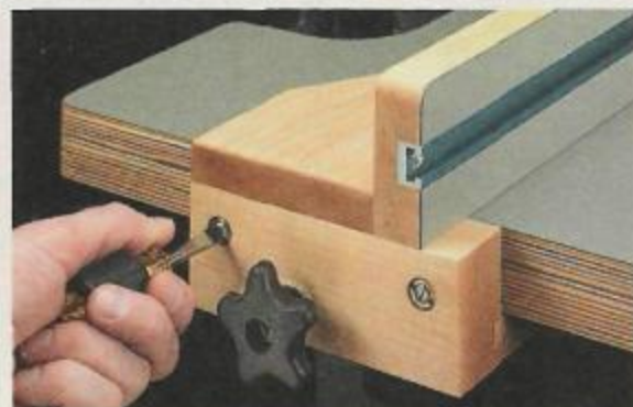
▲ Blade Drift. Adjusting the fence to match the drift of the blade is just a matter of "tweaking" the set screws in the fence.
