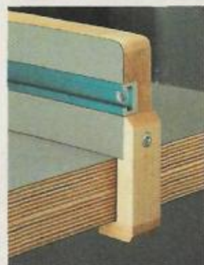
▲ Blade Drift. Adjusting the fence to match the drift of the blade is just a matter of "tweaking" the set screws in the fence.
