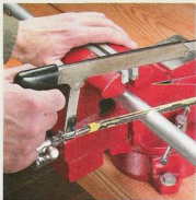
▲ Pipe Jaws. A secondary set of jaws on this vise can be used to hold pipe or rods.
