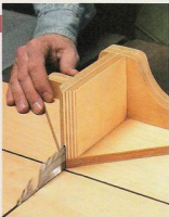
▲ Cutting a Kerf in the Sled. Once the sled is complete, you'll need to cut a kerf. To do this, raise the blade about 1 1/8". Next, push the sled through the blade (left) and complete the kerf by sliding the sled until the blade is "buried" half way into the blade housing (right).
