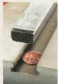
▲ Give the Runners a "Lift." A penny at each end of the metal runner raises it just enough to clear the top of the saw table and contact the base of the sled.
