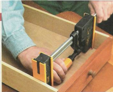
▲ Spread 'Em. Reversing the jaw allows you to use the Gross Stabil clamp as a spreader. (The Jorgensen clamp also has this feature.)
