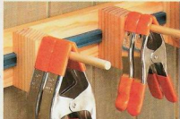
▲ Peg Blocks. By gluing a dowel in an angled hole drilled in a block, you can make a handy place to keep spring clamps. Two peg blocks side-by-side can be used to hold C-clamps in place.
