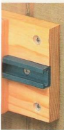
▲ T-Track. Each section of track consists of an aluminum T-track fastened to a wall plate. The sections are then screwed to the wall studs.
