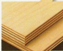
▲ Joinery. Since the plies in Baltic birch are free of voids, traditional joinery and screws make for rock-solid assemblies.
