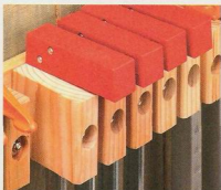
▲ Wide Blocks. To accommodate large, heavy-duty clamps like the parallel jaw clamps shown here, the basic block can be made a little wider.
