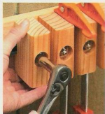
▲ Lock-Down. All it takes to reconfigure the clamp storage system is a ratchet with a 1/16 " socket.
