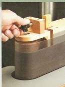
▲ Tracking. Turning a knob at the end of the sander will cause the idler roller to pivot slightly, thereby centering the belt.
