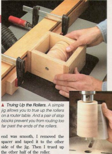
▲ Sanding the Rollers. Each roller is mounted in the drill press and sanded lightly to smooth out the rough surface left behind by the router.
