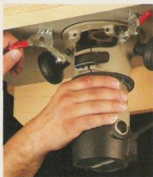
▲ Toggle Clamps. Quick and easy, toggle clamps make it a snap to remove (or install) the router in the table.
