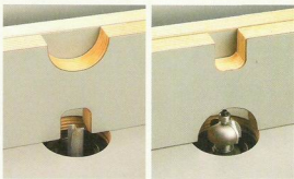
▲ Fence. The front face features two different cutouts so you can match the opening to your bit. The square opening (left) works best for straight bits, while the circular opening (right) provides better clearance for larger profile bits.
