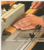
▲ Accessories. An aluminum track allows the use of a miter gauge or the featherboard shown above.
