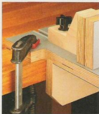
▲ Alternative Mount. You can also mount the router table using clamps on the tabs at the back of the table.
