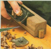
▲ Chamfer Guide. The guide replaces the adjustable throat piece on the plane. Adjusting the size of the chamfer is a simple matter of moving one edge of the guide (left photo).
