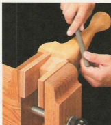
Soft Jaws. For holding delicate objects (like carvings), these leather-lined jaws provide a firm but non-marring grip.
