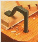
▲ Wedge Action. Striking the top of this iron hold-down causes it to wedge against the workpiece.
