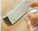
smooth using progressively finer grits of sand paper. After buffing the surfaces with a gray (#00) nylon pad, wipe down the aluminum with mineral spirits then spray on a couple coats of clear lacquer for protection.
