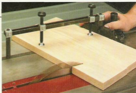
▲ Miter Gauge Hold-Down. The clamp screws on this Delta miter gauge hold-down are adjustable, allowing you to hold either narrow or wide boards for mitering and crosscutting.
