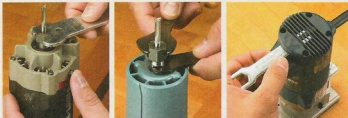
▲ Bit Changes. Like some full-size routers, trim routers that use a single wrench with a spindle lock are common (left photo). But trim routers with dual
