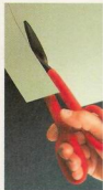
▲ Narrow Strips. Tin snips work great for cutting narrow strips or odd shapes of plastic laminate.
