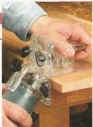
▲ Base Attachment. The attachment shown on the Makita trim router works with the tilting base to rout chamfers with a straight bit.
