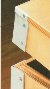
▲ Aluminum Angle. Ordinary aluminum angle reinforces the corners of the gear box. Besides protecting them from wear and tear, the aluminum angle provides a striking look.
