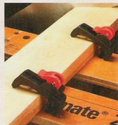
▲ Cam. These plastic-bodied hold-downs use a cam-locking device to apply pressure to the workpiece.
