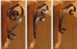
▲ Shelf Brackets. All three shelf brackets shown above were created with the scroll-bending jig. After the metal was bent, holes were drilled and the brackets were screwed in place.
