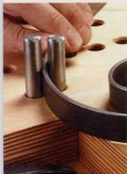
▲ Pins. To create freehand bends, the metal is bent between a pair of steel pins.
