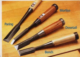
▲ Types of Chisels. Japanese chisels come in a variety of styles depending on their use. Bench chisels (bottom) are designed for everyday work. Long-handed paring chisels (top) are designed for pushing only.
