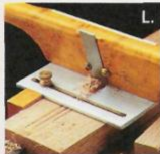
▲ Aluminum. Whether it’s just a piece of flat stock for a stop block (left) or a piece of angle for the body of a shop-made tool like the scratch stock (right), aluminum is easy to use and work with.
