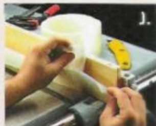
▲ UHMW. Jigs slide easily when they’re guided by a runner (left) made from UHMW. And a workpiece will slide just as easily by adding a thin strip of UHMW (right) to an auxiliary fence.
