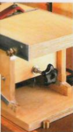
▲ Height Adjustment. Turning a knob at the end of the tapered bed will raise or lower the sliding table.
