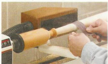
▲ Dust Hood. Hooked up to a shop vacuum, this dust hood does a great job of picking up the fine dust that is created while sanding a project on the lathe.
