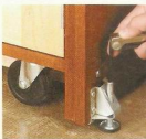
▲ Casters and Levelers – An Allen wrench is all you need to level the stand and raise the casters up off the floor.
