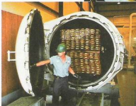
▲ Feeling the Pressure. A stack of freshly-treated lumber is rolled out from a large pressure chamber. Inside the chamber, vacuum pressure is used to impregnate the wood with a liquid chemical preservative.
