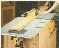
A. Convertible Top. Positioning the top so it extends over the back of the outfeed cabinet creates a long, stable support surface when ripping long workpieces.
