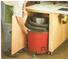
▲ Outfeed Cabinet. Opening the hinged door at the back of the outfeed cabinet provides easy access to the shop vacuum stored inside.
