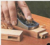
▲ Block Plane. A block plane can quickly trim a rail so it's flush with a stile, either before or after the pieces are assembled.
