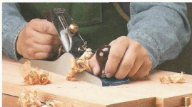
▲ Jack Plane. A jack plane like this #5 can be used to quickly flatten a glued-up panel. Once the panel is level, you can use a smoothing plane (#3 or #4) to remove any planing marks left behind by the jack plane.
