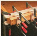
▲ "Stretching" Your Clamps. A couple of cleats attached to the top of the bench allow you to clamp the end apron in place.
