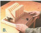
◀ Square V-Block. Slide the alignment plate forward until it contacts all the plates, squaring up the V-block.
