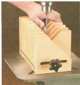
▲ V-Block. The V-block makes it easy to drill a hole in a dowel or round stock. The individual plates of the V-block can be adjusted for different diameters.
