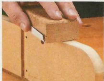
Sand Edges. Make sure the edges of the MDF are smooth by sanding them with 220-grit sandpaper and a sanding block.
