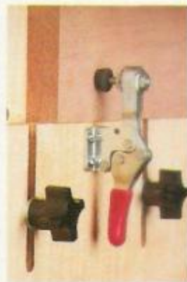
▲ Adjustable. Slots in the sliding plate allow you to adjust the jig for different size workpieces. And a toggle clamp holds the workpiece securely in place.
