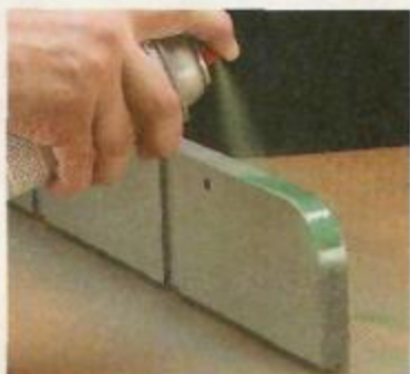
Step 3. Once the primer is dry, you can spray on the hammered finish paint, starting with the edges.
