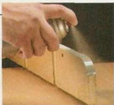
Step 1. Using a gray primer, spray the edges of the MDF first. Apply at least three coats to seal the edges.
