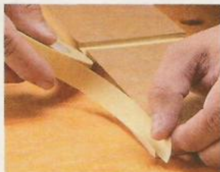
Masking. To avoid getting paint on glue surfaces, mask off all the dadoes, grooves, and rabbets with masking tape.
