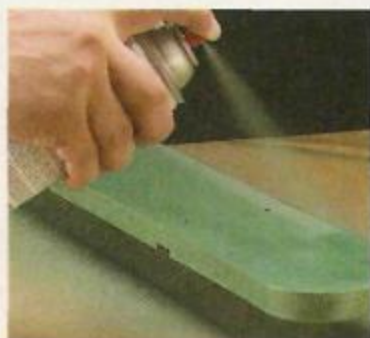
Step 4. In order for the "hammered" finish to work, you have to apply a generous coat of paint.
