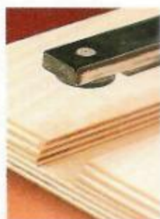
▲ Washer Groove. The washers attached to some miter bars keep it secure in the miter slot. But to store the miter gauge, you'll need to cut a wider groove in your shelf.
