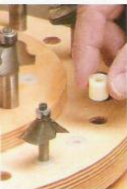
Nylon Bushing. In order to accommodate \frac{1}{4} " shank router bits, a nylon bushing can be used to reduce the size of the hole.
