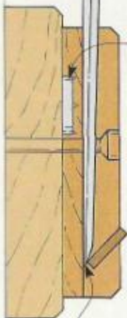
TIP OF CHISEL FITS IN GAP CREATED BY CHISEL REST
