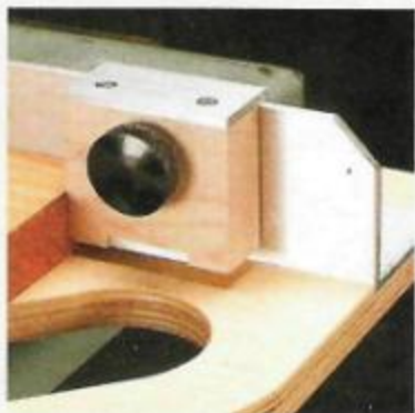
Stop Block. Easy to adjust and rock solid, this stop block makes cutting workpieces to identical length easy.
