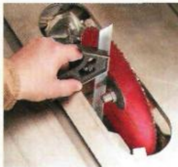
▲ Square the Blade. Using a combination square, check that the saw blade is square to the table.
