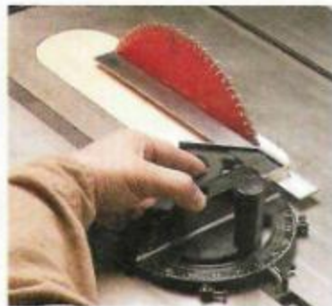
▲ Miter Gauge Check. Finally, adjust the head of the miter gauge so it's square to the blade.
