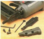
▲ Jam Clearing. Brad nailers that require you to disassemble the nose with an Allen wrench (left) can be a big hassle when you need to clear a jam. But clearing a jam is an easy task on a brad nailer with a quick-release latch (right).
