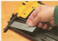
▲ Loading. Loading brad nails is easy and convenient. Just release the magazine, lay a clip inside (above), and then slide the magazine forward to lock it in place.
