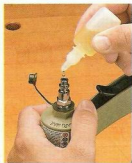
▲ A few drops of oil in the fitting prior to each use will keep your brad nailer firing smoothly each time you use it.
