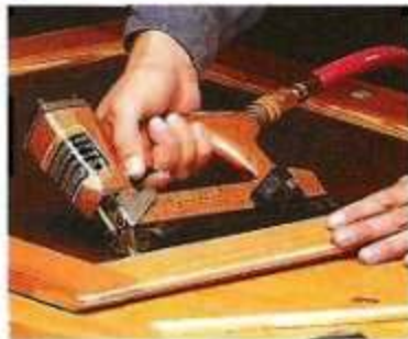
▲ Brad Nailer. Brad nailers and staplers are popular tools with woodworkers as well as carpenters.
