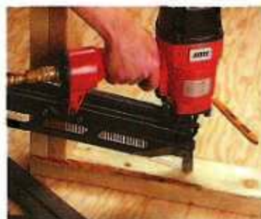
▲ Framing Nailer. Portable compressors can also be used for the occasional framing job.
