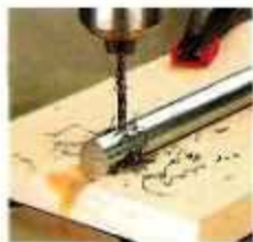
▲ Drilling Round Stock. To drill the cross hole for the cotter pin, hold the axle in a V-shaped block.
