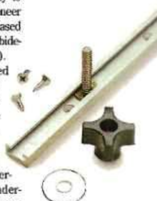
▲ T-Track Hardware. A toilet bolt, washer, and star knob are all you need to clamp an accessory to the T-track. For sources of T-track, refer to page 31.
