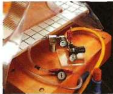
▲ Vacuum Press. A compressor can be used along with a vacuum press for veneering or clamping.
