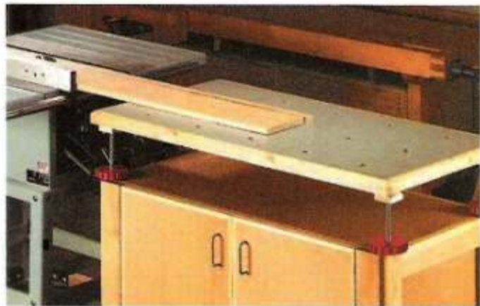
▲ Outfeed Support. Need an extra hand? The assembly table doubles as an outfeed support for the table saw as shown above. Just raise (or lower) the top to match the height of the saw table.
