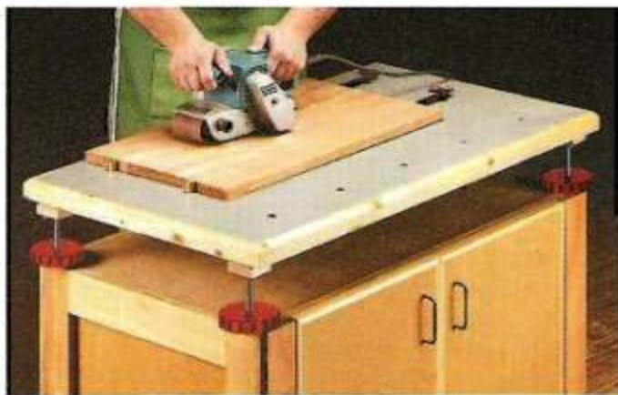
▲ Worksurface. You don't have to use the table just for assembling a project. The top makes a perfect worksurface for a variety of woodworking tasks, like belt sanding a panel flat.
