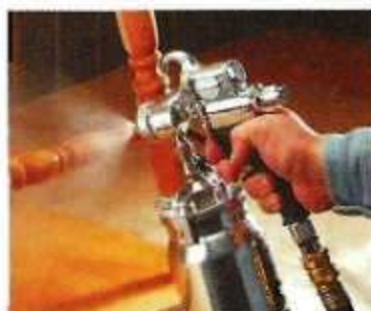
▲ Spray Finishing. Larger compressors will handle a spray gun for applying a perfect finish.
