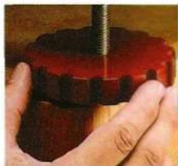
▲ Handwheel. Turning a shop-made handwheel raises (or lowers) the top of the assembly table.
