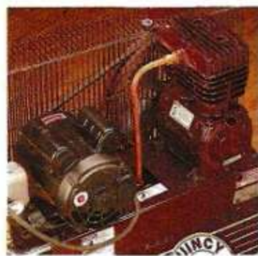
▲ Belt-Drive. A V-belt transfers power from the motor to a flywheel on the compressor pump.
