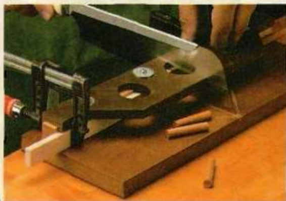
▲ Cutting Dowels. The cutaway at the end of the guide makes it easy to clamp a stop in place and cut small pieces, like the dowels above, to identical length.
