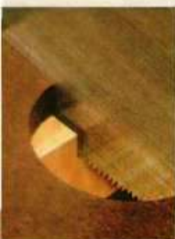
▲ Notch for Teeth. To avoid widening the slot between the guides, the teeth of the saw blade rest in a notch cut in the top of the fence.
