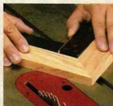
▲ Miter Check. To check the 45° setting on your miter gauge, cut a scrap in two and form a right angle. If it checks square, the 45° setting is accurate.
