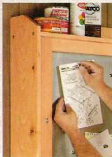
▲ Metal Door. A sheet metal panel is a convenient way to attach plans or pictures using small magnets.
