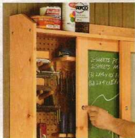
▲ Sliding Doors. Sliding open the doors of the wall cabinet reveals an interior you can customize with shop-made tool holders.
