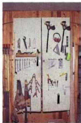
Hand Tool Storage. A wall-mounted storage cabinet provides easy access to commonly-used hand tools.
