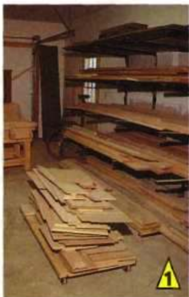
▲ Lumber Storage. A heavy-duty, welded steel rack holds Daryl's supply of hardwood lumber.
