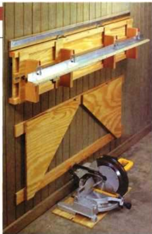
▲ After removing the miter saw, storing the station is just a matter of hanging it on a cleat and folding the supports for the station against the wall.
