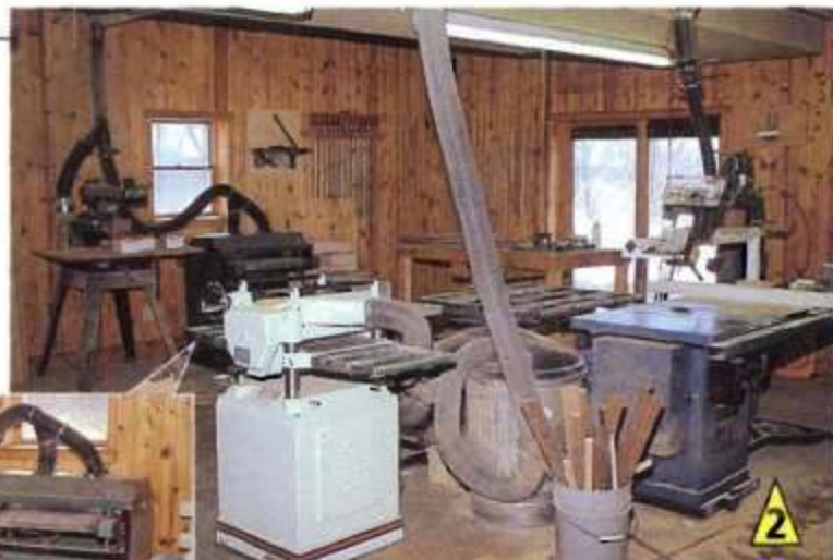
▲ Shop Equipment. A wide belt sander, a 15" planer, and a cabinet saw are some of the big power tools that Daryl uses regularly in his shop.
