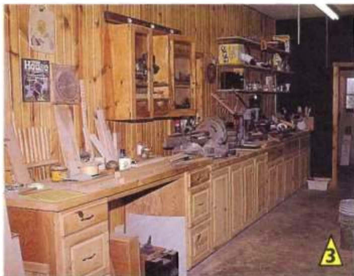
▲ Shop Cabinets. A long bank of shop cabinets provides plenty of storage for hardware and tools. A miter saw station is built into the long work surface above the cabinets.
