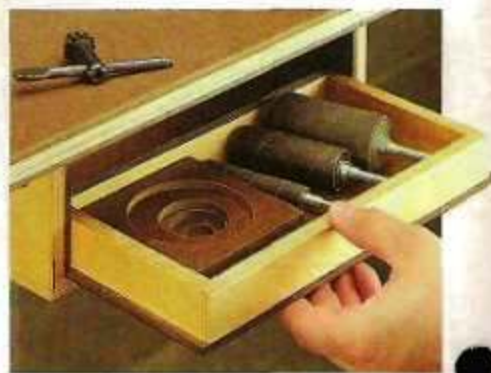
Storage Tray. A small, pull-out tray provides a convenient place for storing a chuck key, drill bits, or sanding drums.
