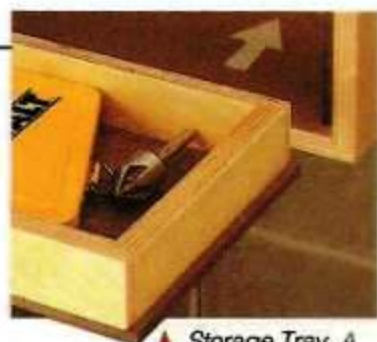
▲ Storage Tray. A shallow tray slides neatly into the base of the drill press table.
