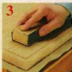
3 Knock Down. Once the wood dries, sand lightly to knock down the raised fibers.
