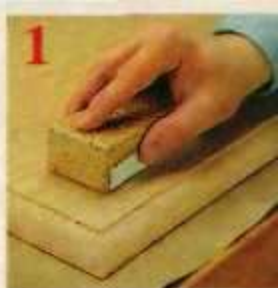
1 Sand. Prepare the surface normally by sanding through a series of grits.
