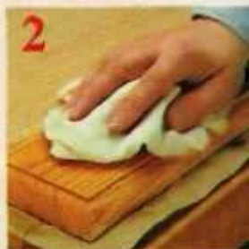
2 Raise Grain. After sanding, raise the grain by wiping it with a damp cloth.
