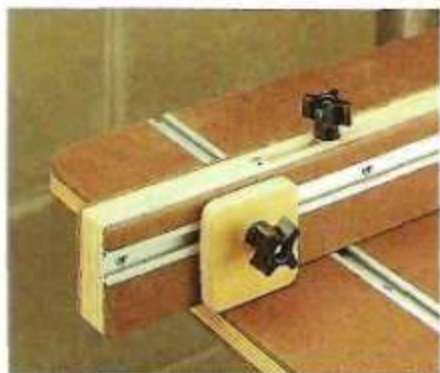
T-Track. Both the fence and the stop block ride in aluminum T-track. Toilet bolts and star knobs are used to lock them in place.
