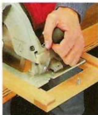
▲ Stop Pin. At the end of a cut, the saw is stopped by a pin in the carriage.
