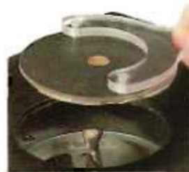
▲ Insert Ring. A spanner wrench is included with the Rout-R-Lift to remove the phenolic ring.
