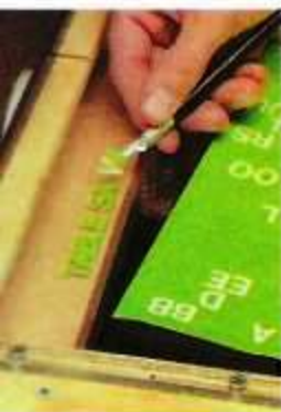
▲ To see which blast gate controls the air flow at each tool, I labeled the front of the box with self-adhesive letters.
