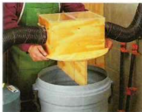
A. Chip Separator. Just lift off the chip separator to empty the trash can. A plastic "window" lets you see when the trash can is full.
