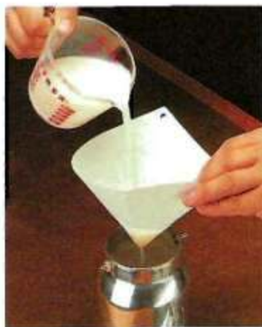
B. Strain the Finish. After thinning the finish, filter it through a strainer to remove any lumps or impurities.
