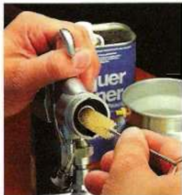
▲ Clean Passages – To clean gunk from the fluid passages, stick a brush inside and work it around.
