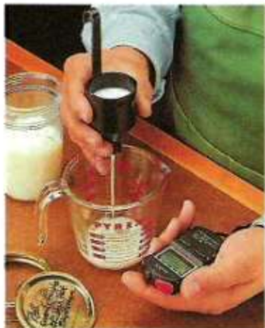
A. Viscosity Check. A properly thinned finish flows through a viscosity cup in a specific time.
