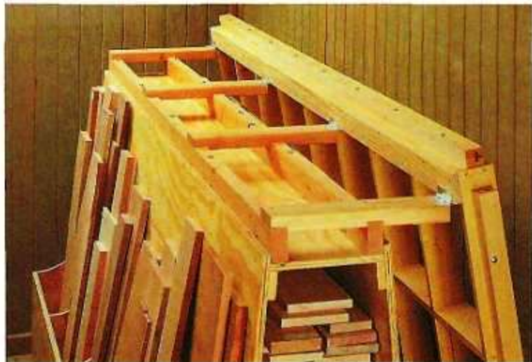
▲ Mounting Assembly. Made of "two-by" material, the mounting assembly for the panel-cutting guide is fastened to the top shelf of the store-all. The guide is hinged to four short crosspieces so it can be tilted out at an angle.
