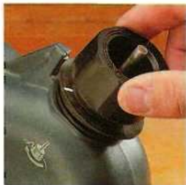
▲ Twist & Sharpen – A few twists of the wrist. That's all it takes when using the Drill Doctor to sharpen a standard twist bit to a 118° point.
