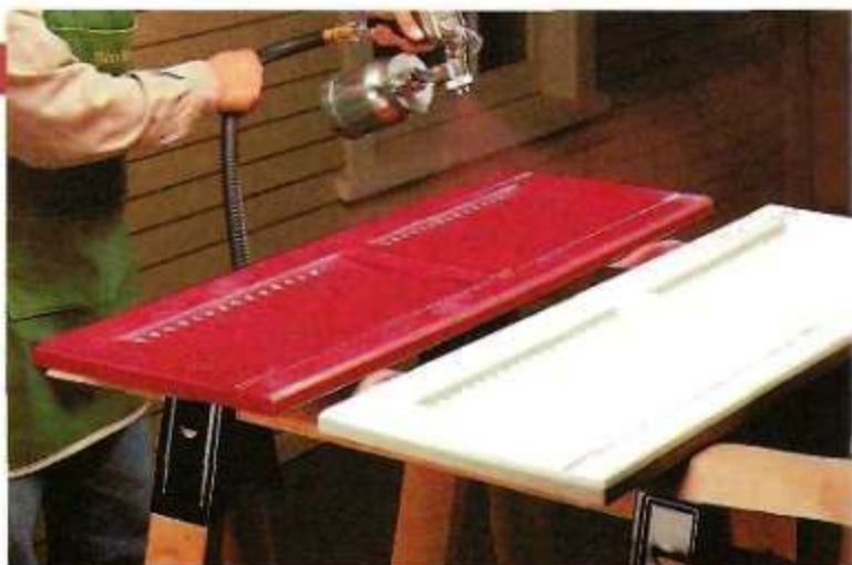
Horizontal Surfaces — When spraying workpieces like these shutters, set them up so you're spraying a horizontal surface whenever possible. Together with a properly adjusted spray gun, this helps minimize drips, runs, and sags.
