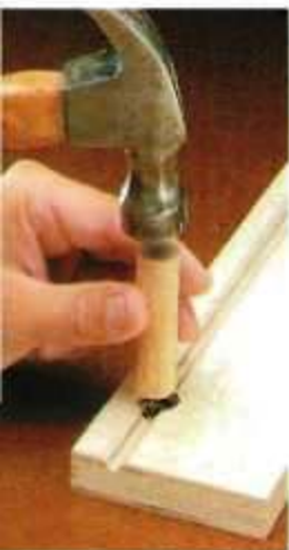
▲ A hammer is too big to fit down into the pocket that holds the T-nut. So I installed the T-nut by tapping a dowel against the head.
