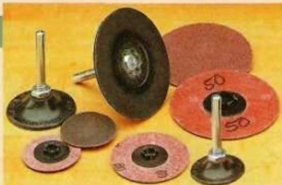
Power-Lock. The locking tabs on these sanding disks snap into a recess in a rubber backing pad. Although it's flexible, the pad is firm enough for minor shaping.
