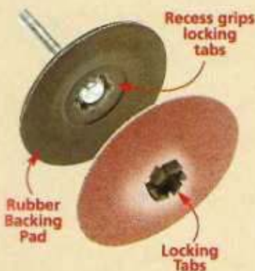
Power-Lock. The locking tabs on these sanding disks snap into a recess in a rubber backing pad. Although it's flexible, the pad is firm enough for minor shaping.
