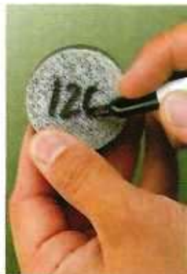
▲ The grit sizes on the sanding disks are hard to see. So to avoid using the wrong disk, I write the grit size on the back with a permanent marker.
