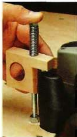
▲ A spring-loaded hold-down "locks" the belt sander in place. To release the sander, simply lift the hold-down and rotate it out of the way.
