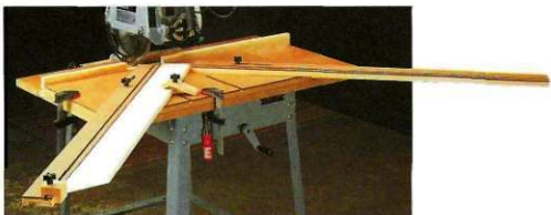
▲ Long Fences. As an option, you may want to build a pair of 48"-long fences to use when mitering extra-long workpieces. With the stop block set at the end of the fence, you can cut pieces up to 46" long.
