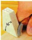
▲ A scrap block cut to a 65° angle provides a handy reminder of the correct cutting angle of the blade.
