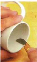
▲ To touch up the edge of a carving knife, run it around the inside of a ceramic coffee cup.
