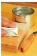
▲ To make it easier to carve hardwood, dampen the surface with water to soften the wood fibers.
