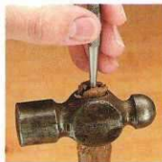
2 To secure the head on the handle, drive the metal wedge below the top of the head.
