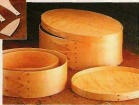
A. Thin Stock. The thin, curved sides of these Shaker boxes are simply resawn from thick stock.
