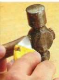
▲ A utility knife is all it takes to trim off the frayed wood fibers at the base of the head.
