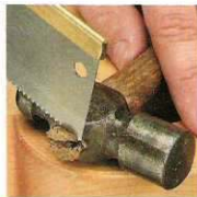
3 Now trim off the waste sticking up above the head. Then sand the end of the handle flush.
