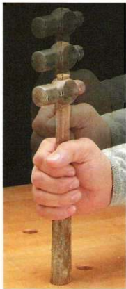
1 To reseat the head of a hammer, start by rapping the end of the handle on a solid surface.
