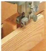
B. Stop/Pivot Block. An adjustable block does double duty as a stop (left) and a pivot block when resawing (right). Tightening a knob clamps the block on the fence.
