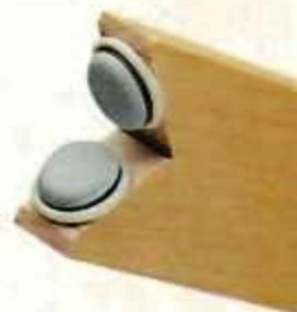
▲ Adding two nylon furniture glides to the notched end of each leg allows the lower support to slide smoothly on the lower rail.
