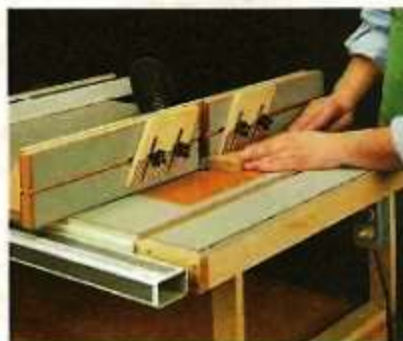
B. Router Table. To save space, the extension table doubles as a router table. There's even a removable fence.
