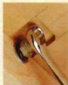
▲ A shallow pocket underneath the table provides clearance for a wrench when installing the mounting bolts.
