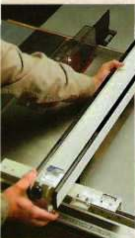
▲ With the fence unlocked, it simply lifts off the guide tube. When you set it back in place, it still locks parallel to the saw blade.
