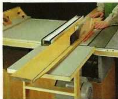
C. Outfeed Support. A simple outfeed table provides plenty of support when ripping a long workpiece.
