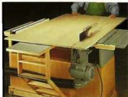
A. Rip Fence. Adding a precision rip fence and a large extension table makes it easy to rip sheet material up to 40" wide.
