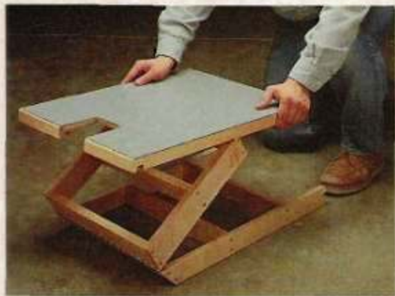
▲ Compact Storage. The outfeed table and ladder-like supports are hinged together. So the entire assembly folds up like an accordion for compact storage.
