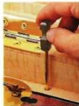
C. Lock System. When closing up shop, slide a brass rod down through the chest (left) to lock the drawers. Then secure the lid with a full-mortise lock and key, see photo at right.
