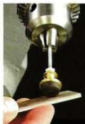
▲ With the knob threaded onto a rod chucked in the drill press, the wood plug is simply filed and sanded to shape. (Two "jam" nuts hold the knob in place.)
