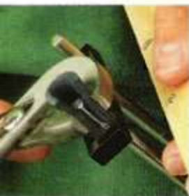
▲ To avoid marring the pins when threading them into the mounting bar, a small piece of rubber is included with the Micro-Fence.
