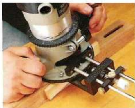
▲ Wide Fence. To rout a mortise with a fixed-base router, attach the wide edge guide. It provides more surface contact with the workpiece as you make a plunge cut.
