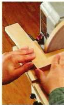
▲ To provide extra support for irreg- lar-shaped pieces, the table extends past the sanding disk.
