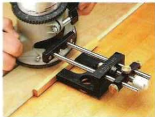
▲ Low-Profile Fence. When the narrow, low-profile fence is mounted to the aluminum body, you can rout a groove (or dado) while the workpiece is clamped flat against a benchtop.
