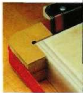
▲ When gluing the apron to the base, a corner block made from scrap protects the fragile tips of the miters.
