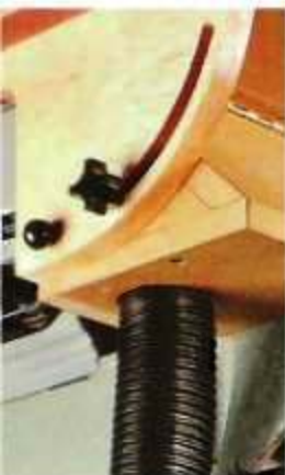
▲ To collect the dust produced by the disk sander, the hose on a shop vacuum fits into a hole in the base.
