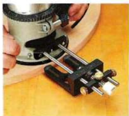
▲ Half-Round Inserts. By mounting pair of plastic, half-round inserts to the aluminum body, you can even rout a groove parallel to a curved edge.
