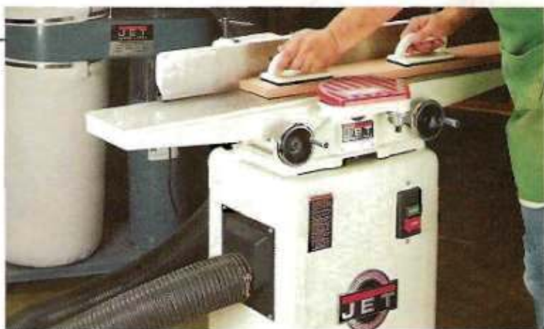
F. Fence. The support on a center-mounted fence sticks out in back, so you can't put the jointer next to a wall.
