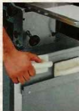
▲ A hardwood strip screwed to the back of the stand provides a handy way to store push blocks.
