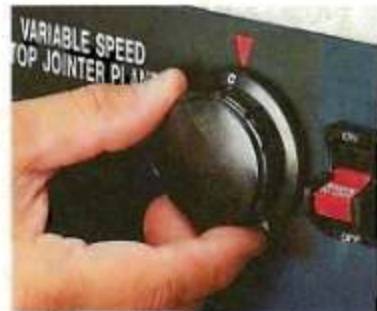
D. Variable Speed. To "dial in" the desired speed on a benchtop jointer, it's just a matter of turning a knob.
