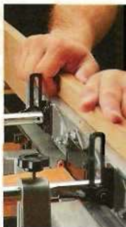
▲ The tall, metal adjustment brackets on this fence are a real knuckle-buster when jointing the edge of a workpiece.
