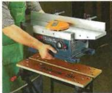
A. Lightweight. A portable jointer is small and lightweight, so it's easy to set up on a temporary work surface.
