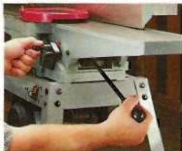
E. Depth Adjustment. Changing the depth of cut is quick with a lever, but it's difficult to make fine adjustments.
