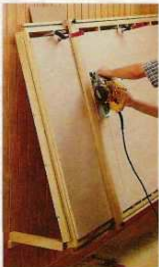
B. Crosscutting. A shorter, vertical fence makes it easy to crosscut sheet goods.
