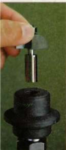
▲ To adapt the 1/2" collet to a router bit with a 1/4" shank, slip a sleeve (included with the collet) onto the bit.
