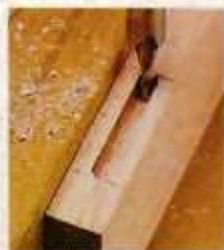
▲ The secret to cutting a crisp, clean mortise is to make a series of shallow passes.
