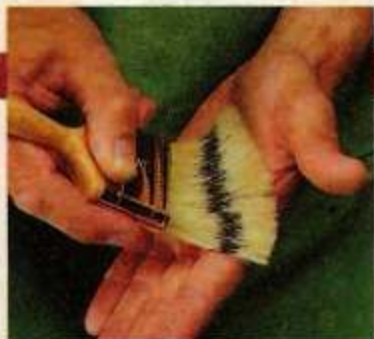
A. Remove Dust & Bristles. Work the brush back and forth in your palm to remove dust or loose bristles.
