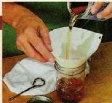
B. Filter Finish. To ensure the finish is clean of dust and debris, filter it into a separate container.
