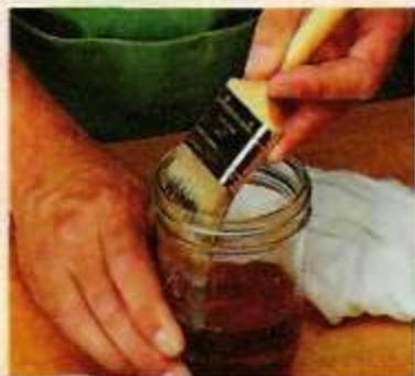
D. Load Brush. After dipping the bristles in the finish, press them against the side of the container.
