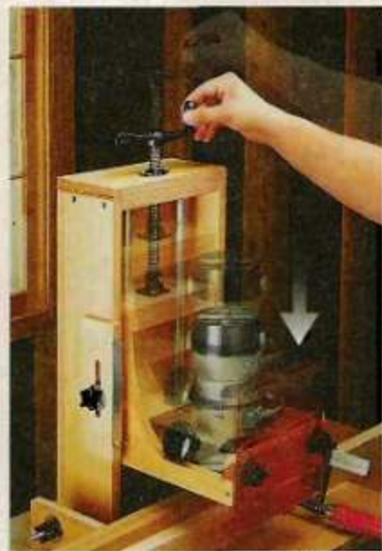
C. Depth. Turning a crank raises and lowers the router carriage and provides control over the depth of the mortise.
