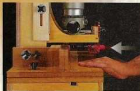
A. Location. It's easy to establish the location of the mortise on a workpiece. Just slide the table in or out to position the piece under the bit.
