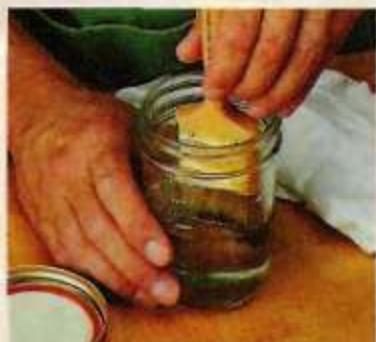
C. Condition Bristles. To condition the brush, dip the bristles into a thinner and then remove the excess.
