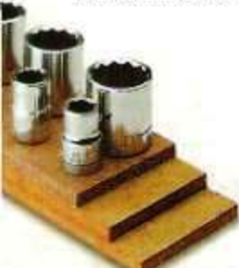
▲ The \frac{3}{8} " sockets are taller, so all you'll need is a pair of \frac{1}{4} " spacers.
