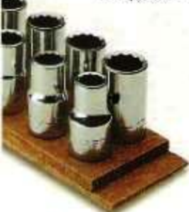
▲ A single, \frac{1}{8} " strip of hardboard builds up the \frac{1}{2} " sockets high enough to "dent" the foam.
