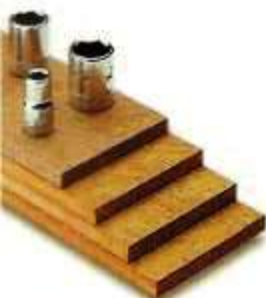
▲ Three \frac{1}{4} " hardboard spacers raise the \frac{1}{4} " sockets just enough to compress the foam in the lid.
