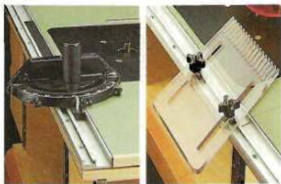
▲ Dual Track. The aluminum track that runs along the front edge of the router table can be used to guide a miter gauge (left) or to attach a featherboard (right).
