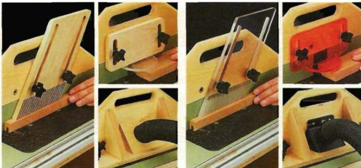
▲ Shop-Made Accessories. A few scrap pieces of material is all it takes to make a featherboard (left), router bit guard (upper right), and a vacuum attachment (lower right).
