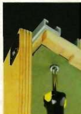
▲ An adjustment screw lets you "tweak" the wings to create a flat, level worksurface.
