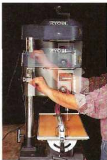
A. Head. The unusual thing about this drill press is you crank the head up and down — not the table.
