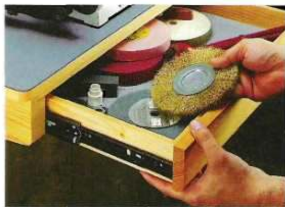
A. Full-Extension Drawer. To provide easy access to accessories, the drawer in this grinding station is mounted on full-extension drawer slides.
