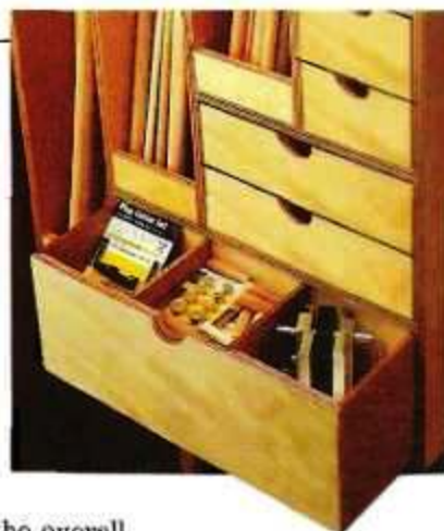
▲ The five drawers are sized to provide a variety of different storage options for your doweling supplies and accessories.
