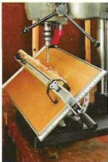
B. Tilting Table. A tilting table and fence make it easy to support round stock or drill angled holes.
