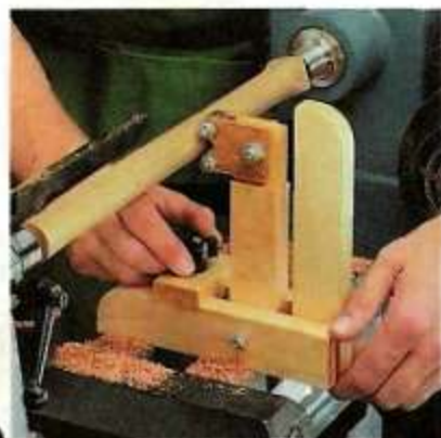
1 To set up the steady rest, slide it forward until the bearings contact the spindle. Then tighten the lock knob.
