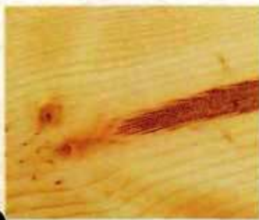
C. Pith. It's the very core of the tree. But you'll find it much too soft to sand and finish.
