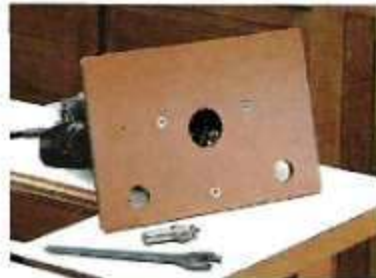
C. Rigid. Phenolic is quite rigid, so this insert plate won't sag when you mount a router to it.
