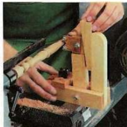
3 To reposition the steady rest closer to where you're turning, slide it along the lathe bed.
