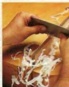
An ordinary hand scraper makes quick work of removing saw marks from a piece of plastic.
