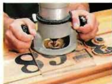
I. Base Plate. An oversized piece of clear plastic makes it easy to see exactly where you're routing.
