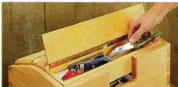
A. Nesting Bins. To provide easy access to small tools or pieces of hardware, a pair of long, narrow bins "nest" in the top of the toolbox.
