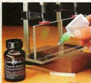
F. Solvent Cement. For a tidy glue job, apply a thin bead of solvent cement with a needle applicator.
