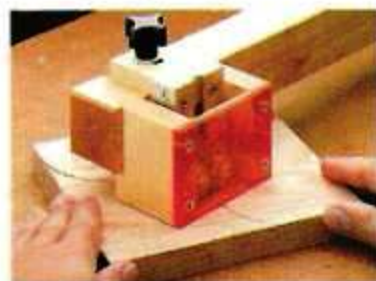
G. Guards. Because they don't shatter, polycarbonates work best for see-through guards.
