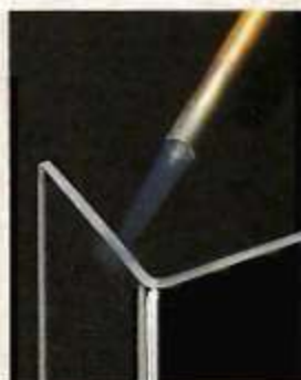
To polish the rough edge on acrylic or polycarbonate, sweep the flame from a torch slowly across the surface.
