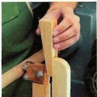
2 Now gently slip the wedge in place. The weight of the wedge applies all the pressure that's needed.
