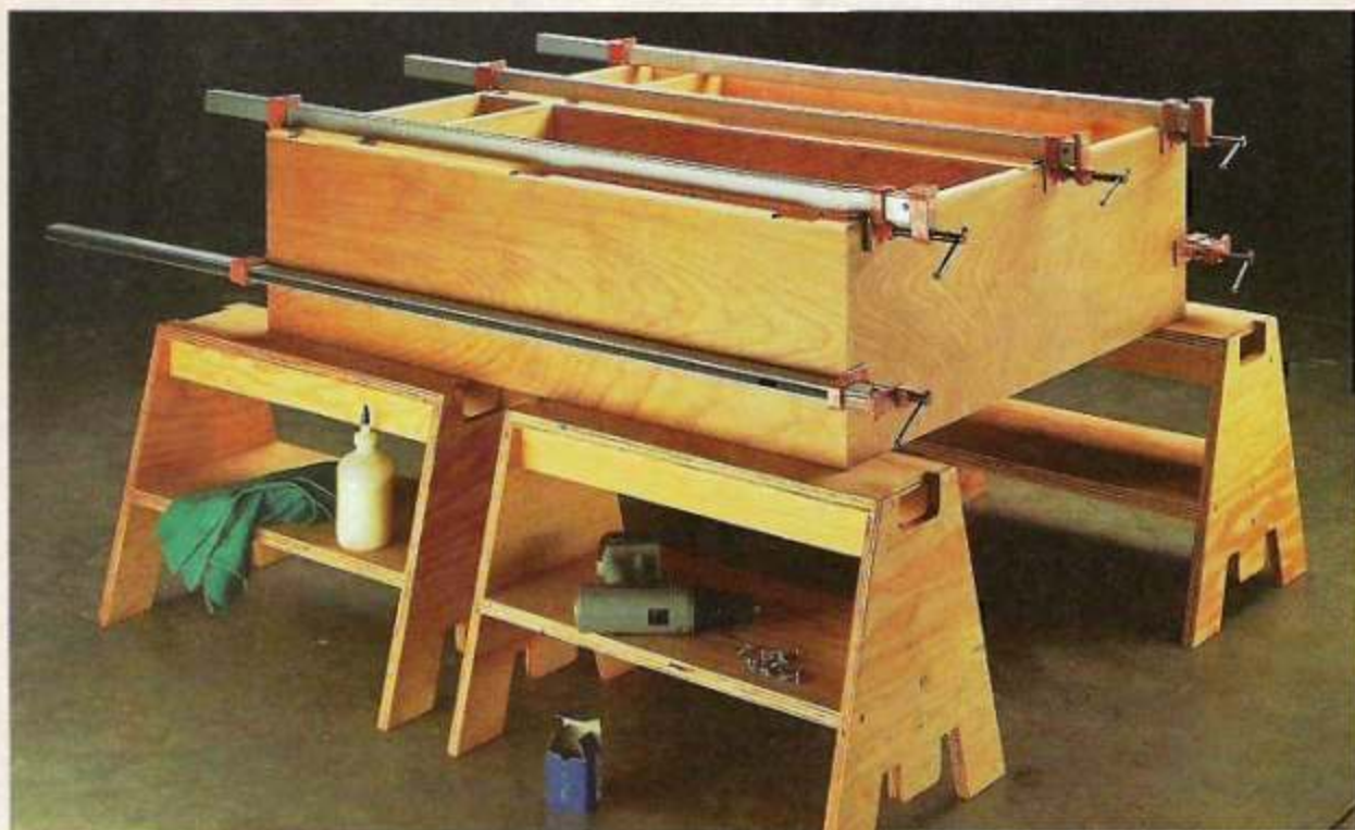
▲ Stacking Sawhorses. Building a large project? This set of four Stacking Sawhorses provides a handy assembly area. Unlike a workbench that's often too tall, in easy reach. And they raise it off the floor so it's not a pain in the back to assemble. (See page 24.)
