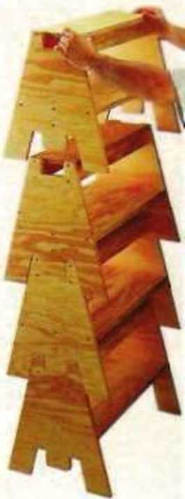
▲ When it's time to "stabilize" your sawhorses, they don't take up much floor space. Just stack all four together for storage.
