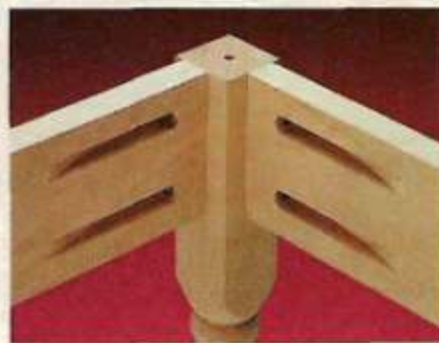
Furniture. After using the jig to cut the pockets in the base of this table, installing screws provides plenty of strength.
