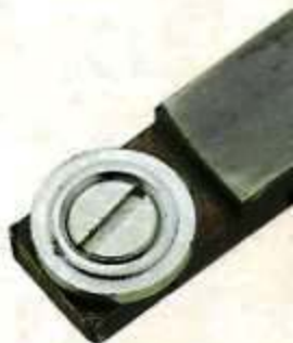
▲ A large washer attached to the end of the miter bar keeps it from falling out of the T-shaped slot in a table saw.
