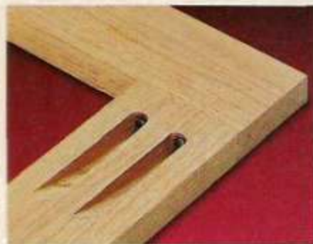
Face Frames. If you're building a face frame, the pocket hole jig makes quick work of joining the rails and stiles.
