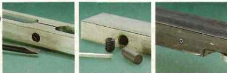
Miter Bars. The adjustment slots in the miter bar of the Osborne (left) are handier than the loose blocks on the Inca (center). Even making a "dimple" produces a snug fit on the Vega and Accu-Miter (right).
