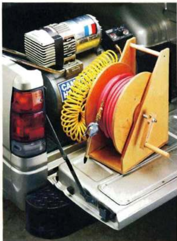
▲ Portable Hose Reel. Helping a friend with a job? Just take your air compressor and this shop-built hose reel with you. (Step-by-step instructions begin on page 6.)
