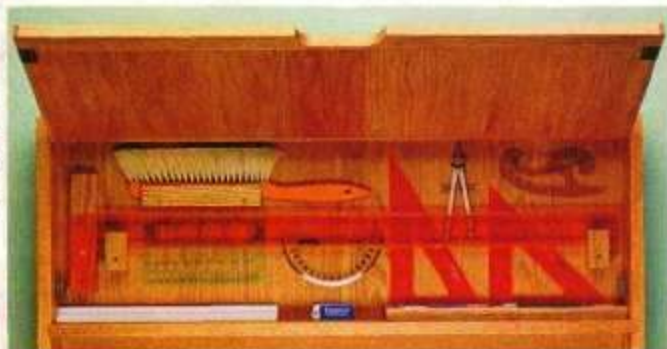
◀ To hold the T-square, the blade is supported at each end by a thick block of hardwood with a kerf in it.
