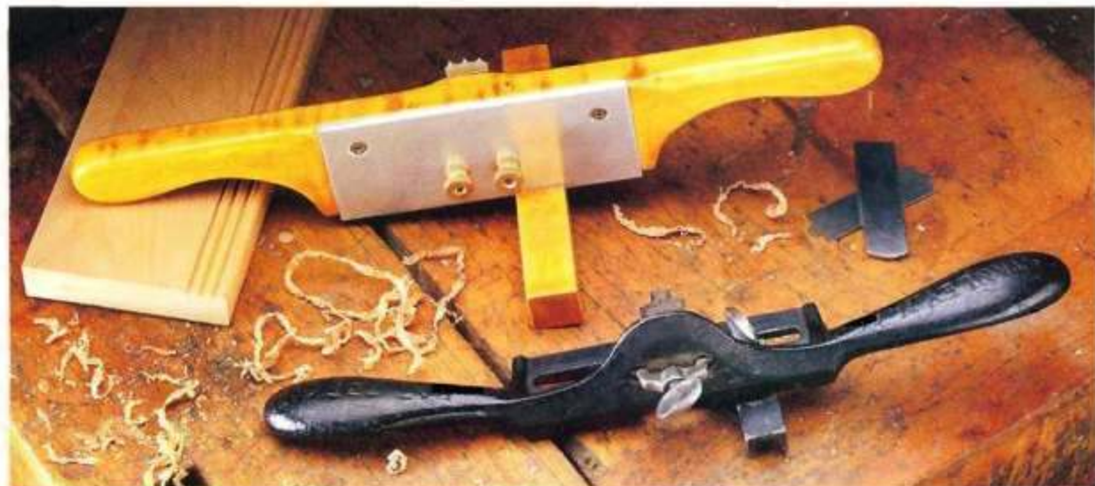
▲ Scratch Stock. The inspiration for our scratch stock (background) came from this old Stanley No. 66 Hand Bearer (foreground). Each tool uses a metal cutter
