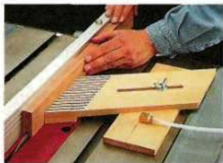
▲ Featherboard. All it takes to attach this featherboard to a table saw is to flip a switch on the vacuum system.
