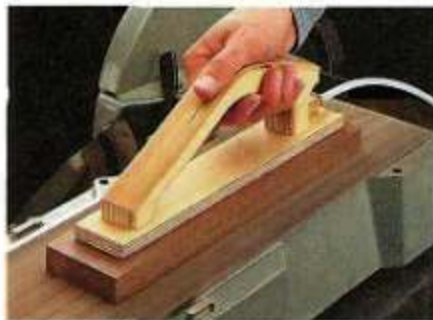
▲ Push Block. This push block works together with the vacuum system to provide a firm grip on a workpiece.
