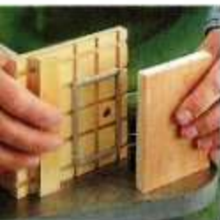
▲ An alignment strip lets you position a workpiece quickly and accurately on the vacuum plate. After applying the vacuum, just set the strip aside.
