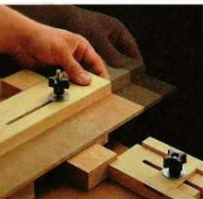
▲ To reduce chipout, just slide the fence in so a small backup block butts up against the workpiece.
