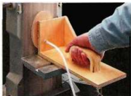
▶ Small-Piece Sanding Jig. A vacuum plate in the front of this jig makes it easy to sand small workpieces safely.
