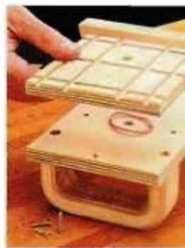
▲ Slipping an ordinary rubber band between the base of the routing jig and the vacuum plate creates an airtight seal.
