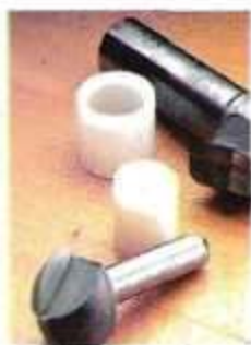
▲ Nylon sleeves make it easy to slip router bits in and out of the drawer.
