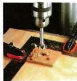
▲ A framing square clamped to the drill press table makes it easy to position the hooks quickly and accurately when drilling holes for the slots.
