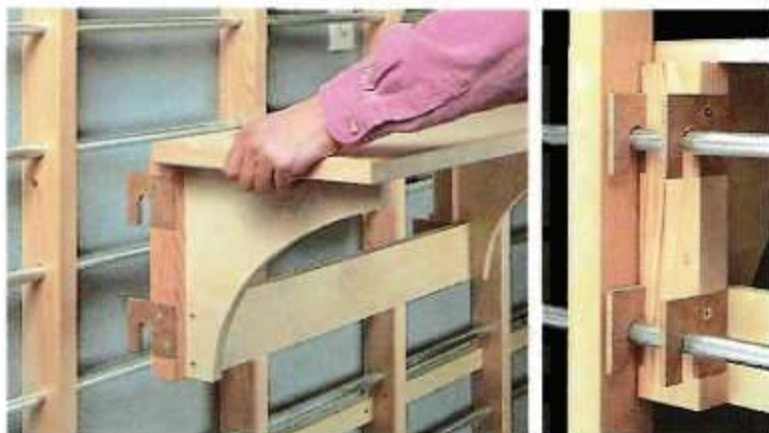
▲ It's easy to hang each storage unit exactly where you want on the grid (left). The secret is a set of hanging brackets attached to the back of each unit that fit securely over the metal conduit (right).
