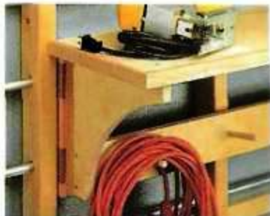
▲ To provide storage under the shelf, glue dowels into angled holes drilled in the stretcher.
