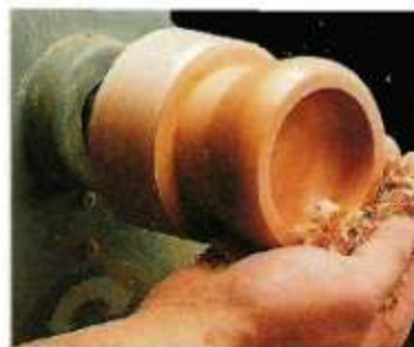
B. Burnishing. To produce a nice sheen, hold a handful of shavings against the workpiece as it turns.
