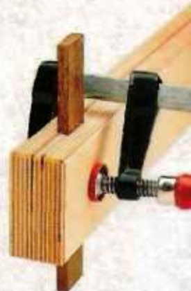
▲ A waxed "key" ensures proper alignment when gluing up the fence pieces.
