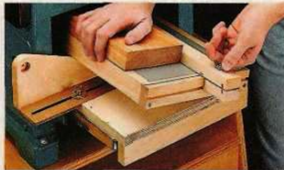
2 After positioning the fence so the workpiece is flush with the edge of the table, it's just a matter of tightening the wing nuts to clamp it to the table.
