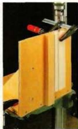
▲ An L-shaped support with a vertical cleat makes it easy to drill a hole in the end of a long workpiece like the adjustment block.
