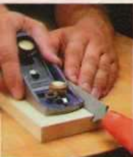
Setting a file in a scrap with a 45° saw kerf makes it easy to create a uniform chamfer on the bottom edges of the plane.
