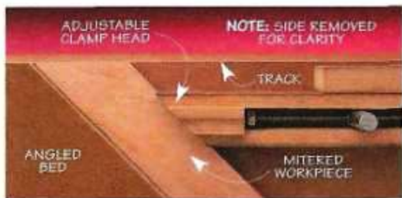
A. Position Workpiece. With the mitered end of the workpiece flush with a track in the top edge, a clamp head presses it against an angled bed.
