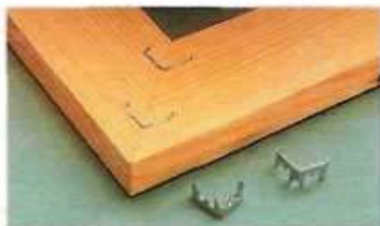
Chevrons. Once these chevrons are tapped in place, the spring steel wings help strengthen the mitered corner.
