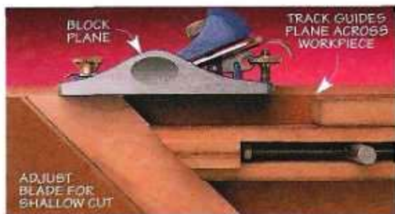
B. True Up End. After adjusting the blade in a block plane for a very light cut, slide it along the track and across the workpiece to true up the end.
