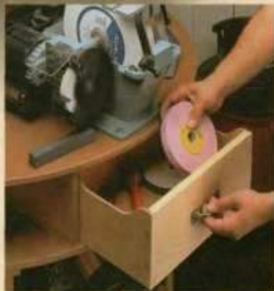
B. Drawers. With a drawer below each tool, there's plenty of storage for accessories and other items.
