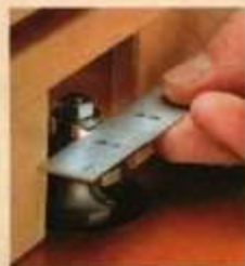
A With a metal rule held on edge, it's easy to align the fence so it's flush with the bearing.
