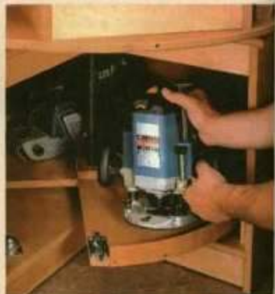
C. Turntable. A spin of the turntable in the base provides quick and easy access to portable power tools.
