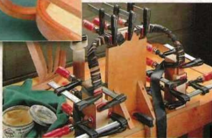
B. Compound Curve. To create a compound curve, the wood strips are bent and twisted around a jig to form a dramatic bent wood shape.
