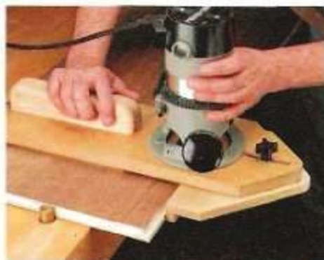
Edge Guide. By replacing the stop with a triangular-shaped edge guide, you can rout rabbets quickly and accurately with an ordinary straight bit.
