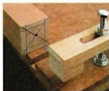
Step 1. After laying out the tapers on the end of the leg, drill a centered hole to fit on the pin.
