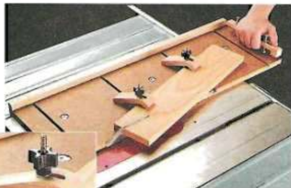
Angled Cuts. Two adjustable hold-downs clamp work securely in place when making angled cuts.
