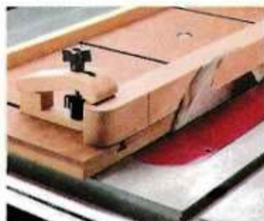
Step 6. After cutting a taper on one side, rotate the leg and repeat the process for each side.
