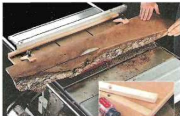
Ripping. To rip a straight edge on a rough board, just remove the runner.
