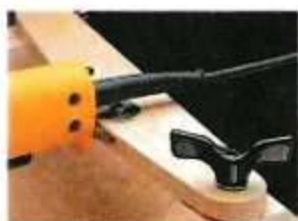
With some plate joiners (like this DeWalt), you'll need to position the arm below the power cord.
