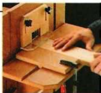
An adjustable stop and blade guard provide safer cuts — especially when cutting a slot in end grain.
