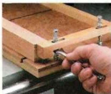
Step 2. With the leg in place, adjust the hex nuts up or down so it sits flat on the platform.
