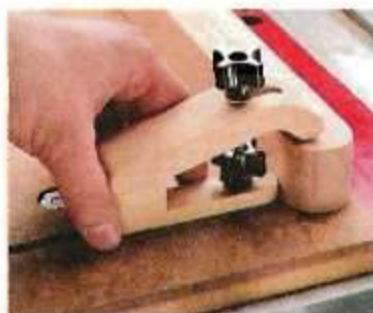
Step 5. Slide the stop against the leg and lock it in place. Then tighten the hold-down on the leg.
