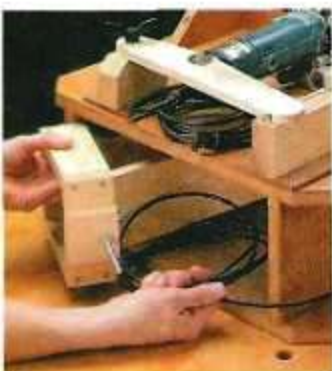
When you're not using the plate joiner table, just slide the foot pedal into the opening at the back of the base.
