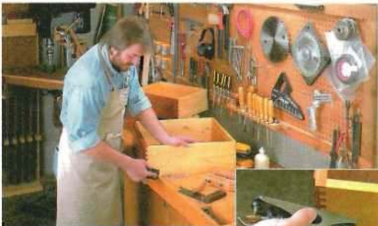
▲ Using his low-angle Record block plane, Steve Curtis (our shop manager) trims the pins of a dovetailed drawer.
