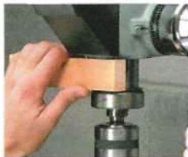
Step 2. Before attaching the arm, use a 1½" tall (wide) block to temporarily hold the quill down.
