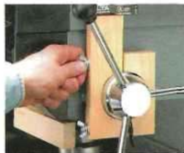
Step 3. Position the pinch block straight up and down and tighten it around the hub of the feed lever.
