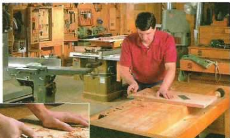
▲ Steve Johnson (our shop craftsman) chamfers the end of a glued-up panel with his Lie-Nielsen low-angle block plane.
