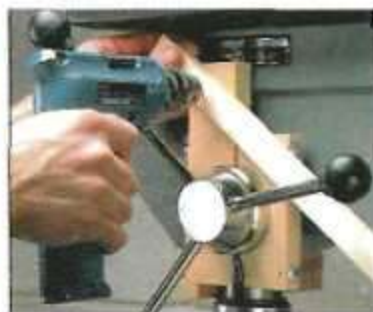
Step 5. After drilling a hole in the top end of the arm, cut it to length and attach it to the pinch block.
