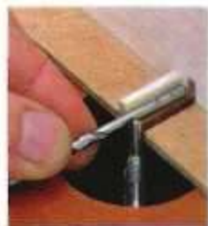
An \frac{1}{8} " drill bit makes a handy gauge to help position the key.
