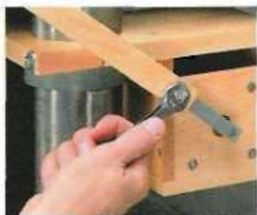
Step 4. Now bolt the arm to the crank and align the two parts as shown here and in Side View.
