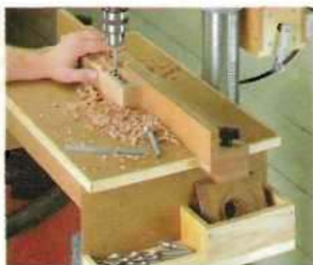
C. Fence. A simple fence with a built-in clamping system also lets you use the sanding platform as a drill press table.
