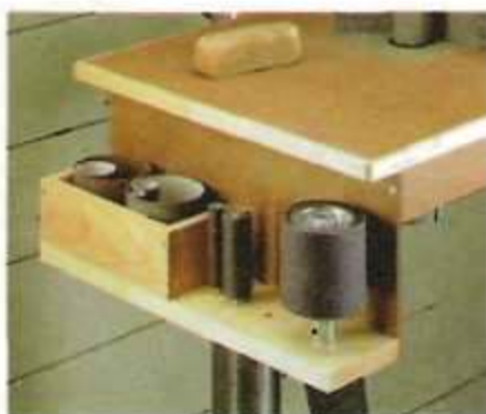
B. Storage. Keep your sanding (or drilling) supplies in easy reach with a storage rack on each side of the platform.
