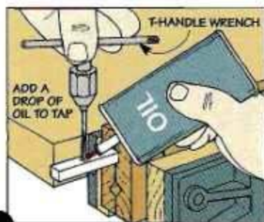
Step 4. Now position the tap so it's straight up and down and add a few drops of oil.
