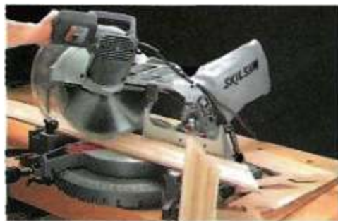
Crown Molding. Finally, we cut compound angles on pieces of crown molding and fit them around the top of a simple cabinet.
