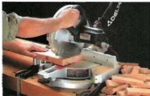
Crosscutting. To get a feel for the basic crosscutting operation and controls of each saw, we cut stacks of "two-by" material.
