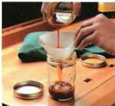
B. Strain. After the shellac is completely dissolved, strain it through an ordinary paint filter.
