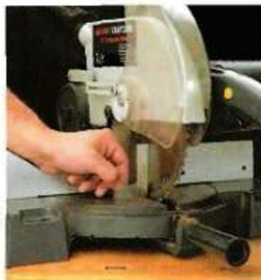
A. Set 0° Stop. After adjusting the 0° stop so it contacts a casting on the arm, align the indicator to the 0° mark on the bevel scale.
