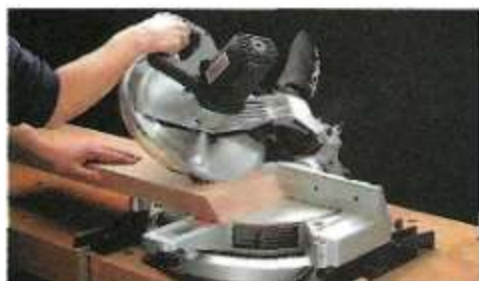
Bevels. Cutting bevels in 2"-thick oak gave us an idea of the power of the saw and whether the blade deflected in a heavy cut.
