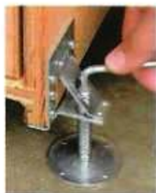
Use an Allen wrench to adjust each leveler and raise the miter saw station off its casters.
