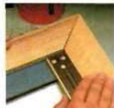
Now form a "corner" with the two cutoffs and check it for square.
