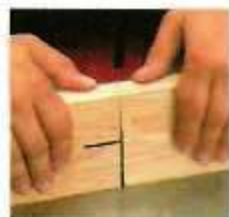
Now flip one of the cutoffs over and butt the pieces end to end to see if there's a gap.
