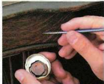
Repairs. Shellac is compatible with most finishes, so it's ideal for repairing damage. Just use shellac that's close in color and dab it into the scratch.
