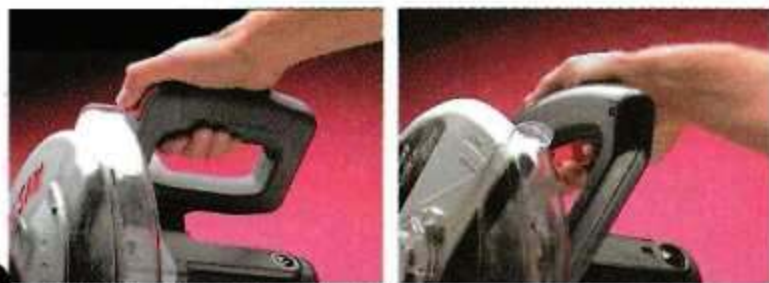
Handles. A horizontal handle (left) is more comfortable to use than a vertical handle (right). But regardless of the style of handle, the safety switch on the Skil (left) and Sears (right) are awkward to use.
