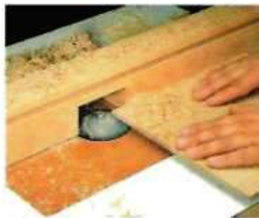
Raised Panels. To see how the routers perform when mounted in a table, we routed raised panels.
