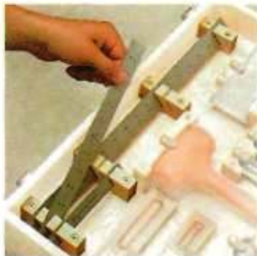
▲ Small turnbuckles made of walnut prevent tools from falling out. To slip easily over the tool, you may need to sand a slight bevel on the end.
