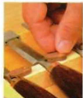
▲ Small turnbuckles made of walnut prevent tools from falling out. To slip easily over the tool, you may need to sand a slight bevel on the end.
