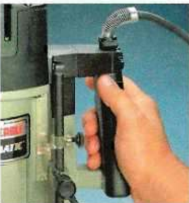
Handles. The handle on the Hitachi (left) adjusts to provide a comfortable grip. And it's attached in just one place. So it doesn't "trap" your hands like the dual supports on the handle of the Porter Cable (right).
