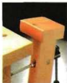
To hold carving blocks securely in place, you can glue leather strips to each clamping surface.
