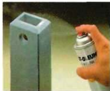
Step 4. Finally, spraying on an acrylic clear coat helps to protect the painted finish.
