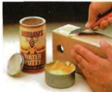
Step 1. To prevent the edges from absorbing paint, fill them with putty, then sand them smooth.
