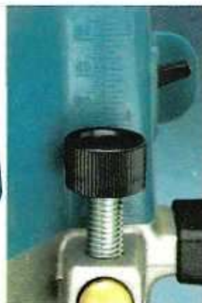
Scales. The depth of cut scale on the Makita (shown here) and the Ryobi are hard to read. And there's no hairline indicator for setting the depth of cut accurately.
