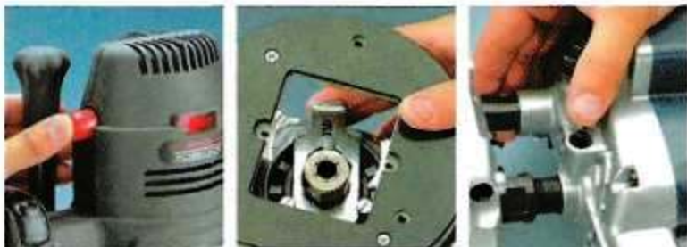
Spindle Locks. A sliding bar on the Sears (left) locks the spindle and leaves both hands free to change bits. So it's more convenient than a spring-loaded "wrench" (center) or button (right).
