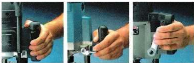
Plunge Lock. The plunge lock switch on the Sears (left) and the lever on the Makita (center) are easy to use. But you have to unlock the lever on the Porter Cable (right) to make a cut — and that's a nuisance.
