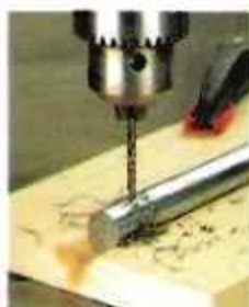
To make a cross-dowel, drill progressively larger holes (up to \frac{7}{16} " in a steel rod that's clamped in a V-shaped block.
