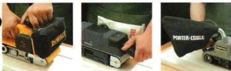
Dust Collection. The dust bag on the DeWalt (left) is small and out of the way. But it doesn't collect as much dust as the side-mounted bag on the Bosch (center) and the Porter Cable's rear-mounted bag (right).
