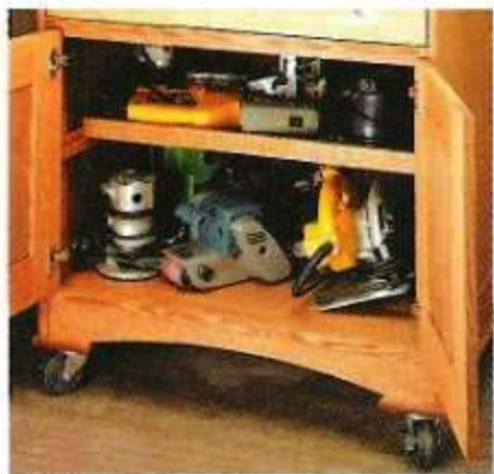
B. Shelf & Tray. Portable power tools are stored underneath on a large bottom shelf and a sliding tray.
