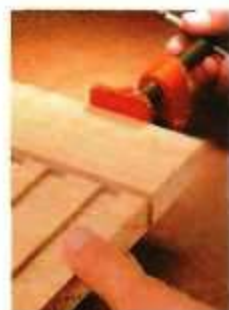
Cutting stopped dados is easy. Just cut the front edge off the panel. Then cut a series of through dados, and glue the front edge back in place.
