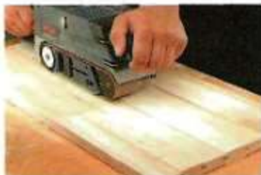
Panels. To test whether the motors would bog down on a tough job, we sanded glued-up panels flat.
