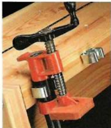
A. Storage Rack. A simple metal broom clip helps secure each pipe clamp for storage.
