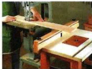
C. Overlapping. Take advantage of different table heights by overlapping infeed/outfeed areas.
