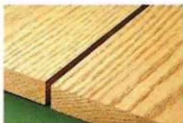
Straight Grain. Positioning one straight-grained board next to another creates an "invisible" joint.
