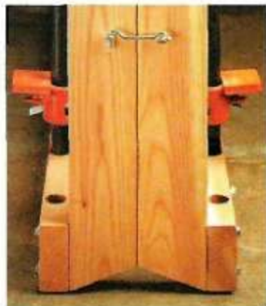
C. Compact Storage. When folded for storage, the glue-up station requires very little floor space.
