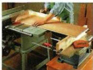
A. Support. A board clamped to the fence of the jointer provides support for a long workpiece.
