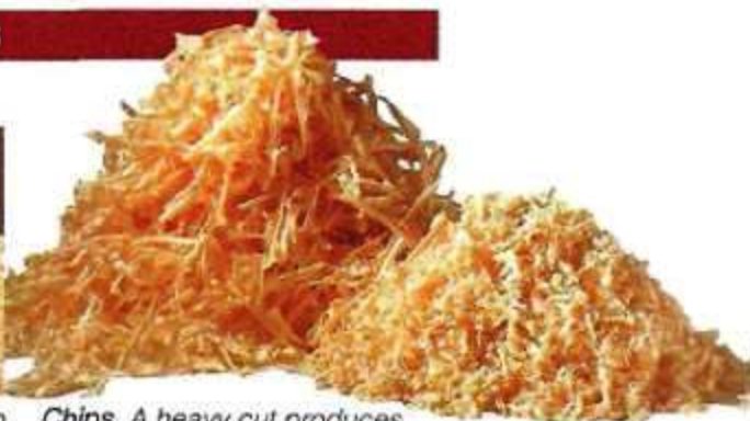
Chips. A heavy cut produces thick chips (left) and a rough surface. But you get fine shavings (right) and a smooth surface with a thin cut.
