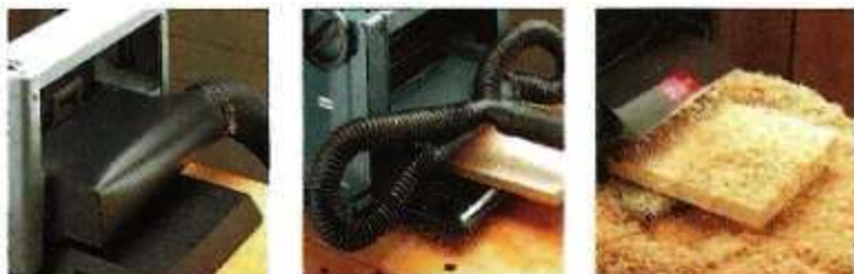
Dust Hoods. A single port on Delta's dust hood (left) doesn't clog up during a heavy cut like the dual ports on the Jet (center). With no dust hood, the Sears (right) throws chips everywhere.
